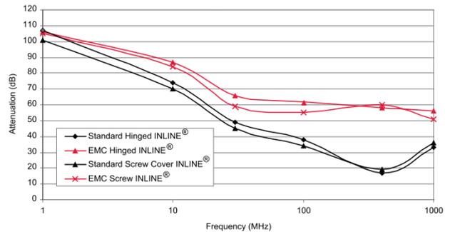
**Figure 3. Hoffman INLINE<sup>®</sup> Hinged Cabinet Shielding Effectiveness Standard Cabinet Compared to EMC Shielded Cabinet (see Appendix – Noise Mitigation Solutions).**
